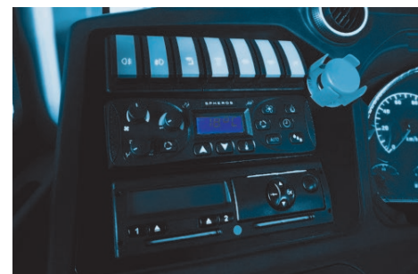
SC 1000 – integral control unit at the driver’s seat – for worldwide use.
