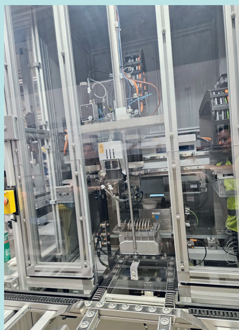
Glue dosing station
