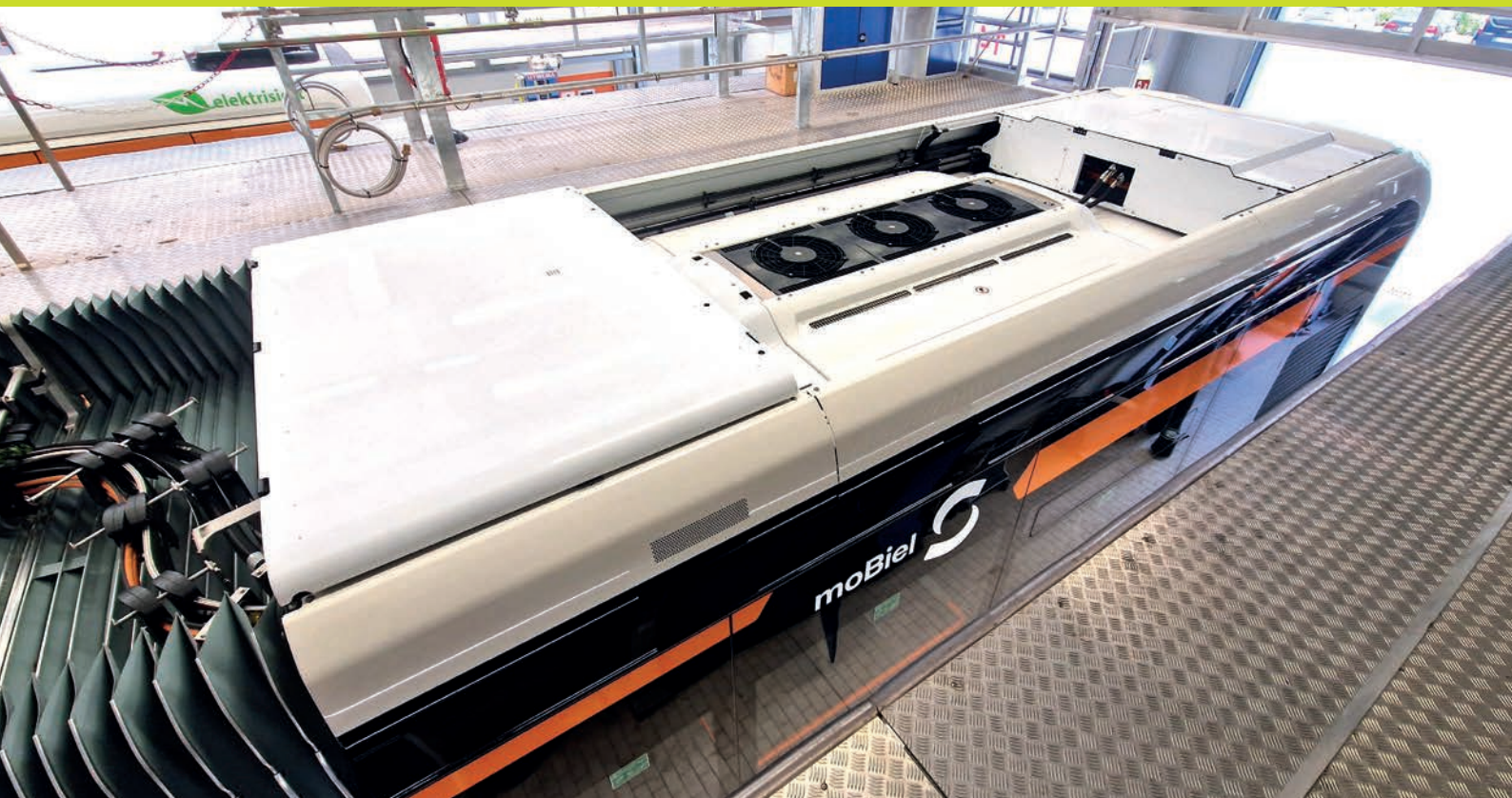
View of the bus roof with the Spheros REVO® HP air conditioning system with heat pump technology.
