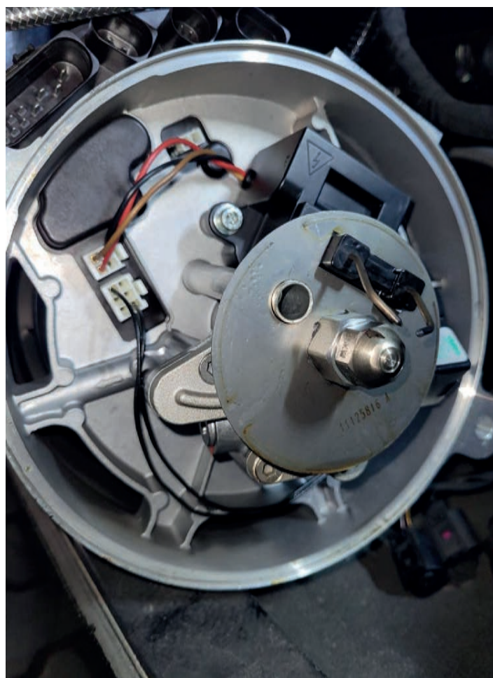
Opened burner head of a Thermo plus 300 CAN after an operating time of 9 months with HVO100 – free of deposits.
