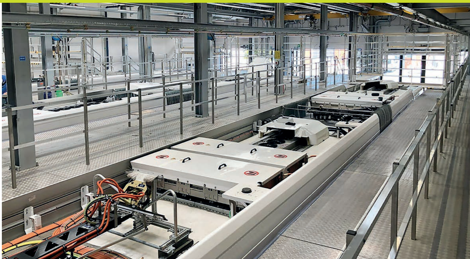
View of the electrical components on the roof of an electric articulated bus.
